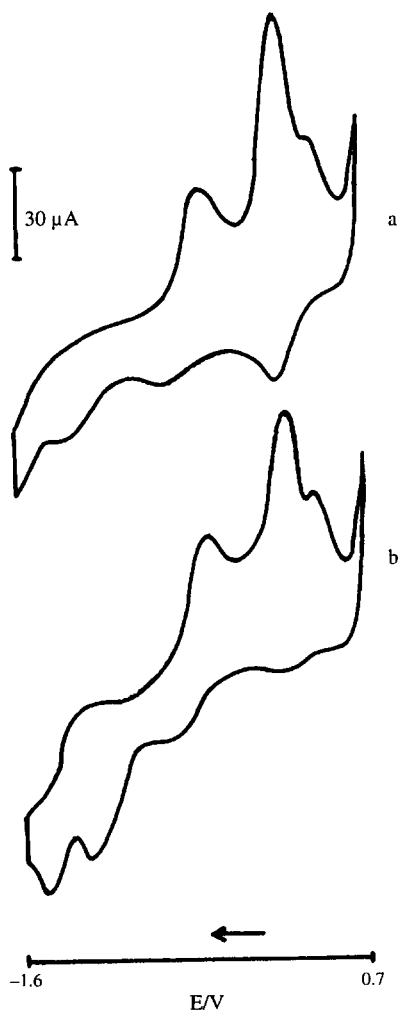
Fig. 7. Cyclic voltammograms for the complexes (a) [\text{Cu}(\text{H}_2\text{L}^2)(\text{H}_2\text{O})_2]\text{Cl}_2 ; (b) [\text{Cu}(\text{H}_2\text{L}^5)(\text{H}_2\text{O})_2]\text{Cl}_2 ; in DMSO (0.1 M TBAP); scan rate = 100 mV.
